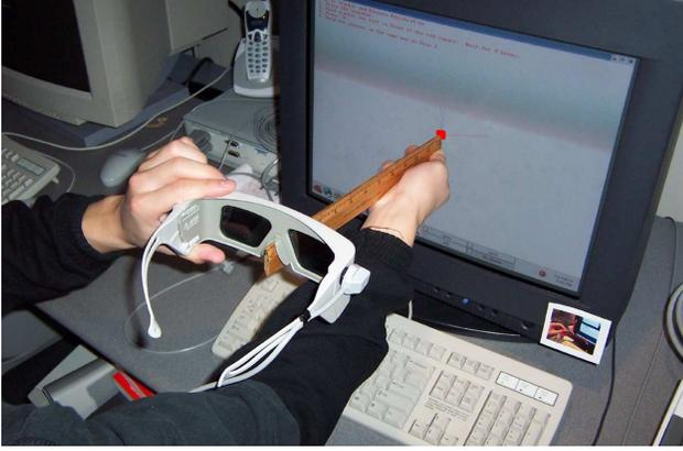
Figure 4: The pose used for registering the tracked glasses is similar to that for basic registration. The point midway between the viewer's eyes is positioned in the same known point, and the glasses' lenses are oriented parallel to the display.
