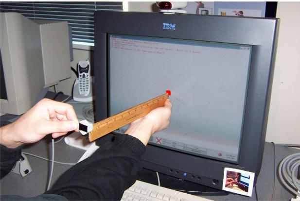
Figure 3: To do the basic registration, a tracker is oriented such that its local coordinate system is aligned with the display's coordinate system, and it is positioned at a known point relative to the display. The red marker, emphasized here for clarity, indicates the position of the known point projected onto the display. The small image attached to the lower-right of the monitor is a picture reference that we used in our study, to help users understand the tracker's local coordinate system.
